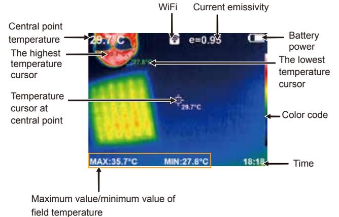
Color code: used to mark the color corresponding to the relative temperature from low to high in the field of version.
