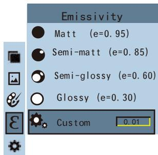
As shown in the figure, press " ⏏ / MENU " key to enter the main menu and select " Ⓔ "(emissivity) option and press " ▶ " key to enter the emissivity list.
