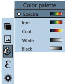
As shown in the figure, press “ $\mathcal{O}$ /MENU” key to enter the main menu and select “ $\mathcal{C}$ ” (color palette) option and press “ $\blacktriangleright$ ” key to enter the color palette list. Press “ $\blacktriangle$ ” and “ $\blacktriangledown$ ” keys in navigation to select the color palette. Then press “SELECT/ENTER” key to select the color palette. Press “ $\blacktriangleleft$ ” to return. Press “ $\mathcal{O}$ /MENU” key to exit from the menu.
